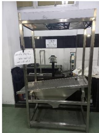
**Gambar 4.1** Design mesin *vibration table*
