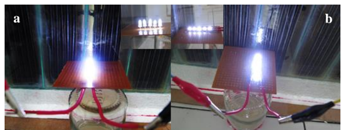
Fig 10. Lighting of five LED lamps (a) white DIP LED, (b) high power LED
