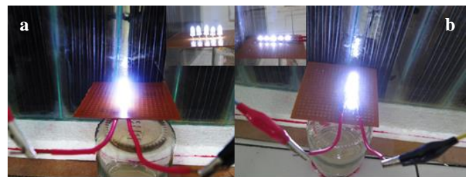
Fig 10. Lighting of five LED lamps (a) white DIP LED, (b) high power LED
