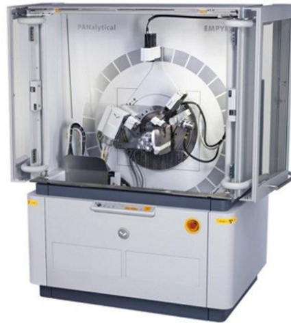
Gambar C.1 Mesin XRD Empyryan Panalytical
