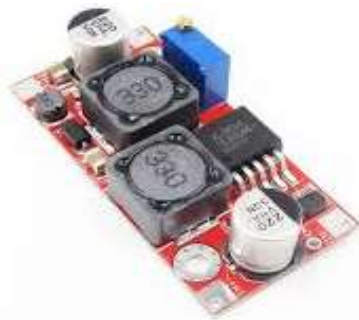
Gambar 2.8 Modul Konverter DC to DC Step Down
