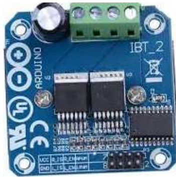
Gambar 2.3 Motor Driver BTS7960 [18]
