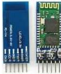
Gambar 2.4 Modul Bluetooth HC-05 [20]
