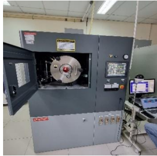
Gambar C.1 Spark Plasma Sintering (SPS) Fuji SPS-625
