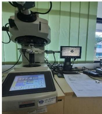
**Gambar 3.10** *Micro Vickers Hardness* HM-200
