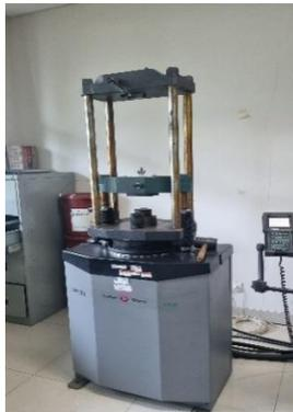
**Gambar 3.11** Alat *Universal Testing Machine*
