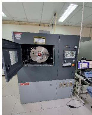
**Gambar 3.2** *Spark Plasma Sintering* (SPS) Fuji SPS-625
