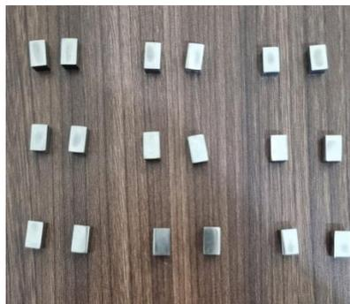
**Gambar 3.5** *Wire Cut* Hasil Proses SPS
