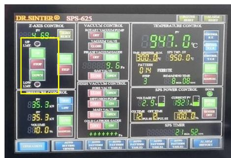
**Gambar 3.3** Spark Plasma Sintering Monitor Controlling
