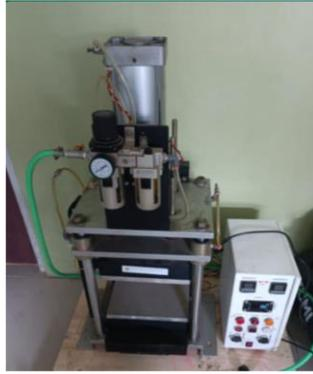
**Gambar 3.2** Mesin *Hot press*
