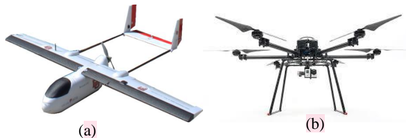
Gambar 2.1 Jenis UAV (a) fixed wing , (b) rotary wing
