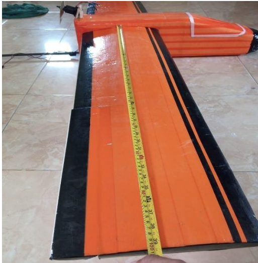
Panjang Half Wingspan 100cm
