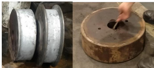
Gambar 4.4 Roda Car Mesin Shot Blast (Sumber: Cold Rolling Mill PT. KPdP)
