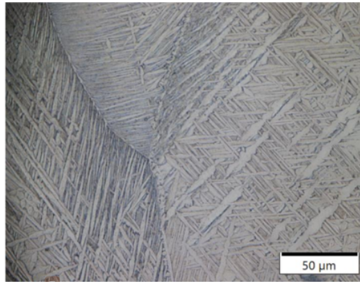
Gambar 4.2 Struktur mikro as-cast paduan Ti-6Al-5Nb-3Zr-1Sn
