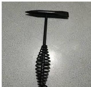
**Gambar 3.11** Spring Welding Hammer
