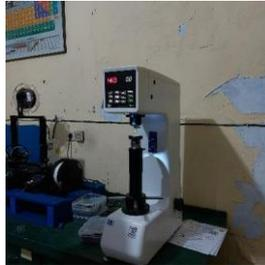
**Gambar 3.19** Alat Uji Kekerasan Rockwell
