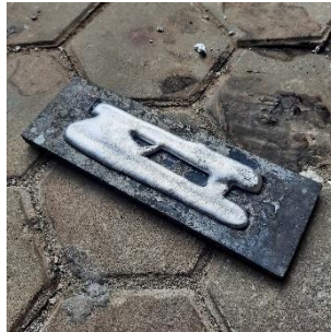
Gambar 3.37 Hasil proses stir casting
