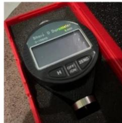
**Gambar 3.3** Durometer Shore-D
