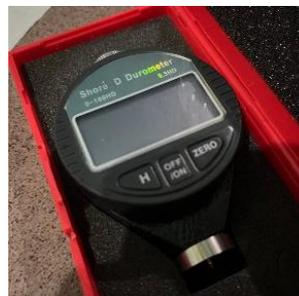
**Gambar 3.3** Durometer Shore-D
