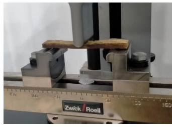
Gambar 2. Proses Uji Bending
