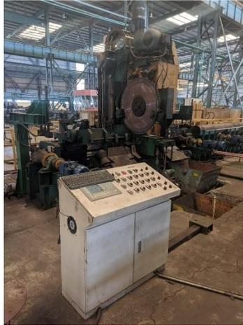
**Gambar 3.2** Mesin *Pipe Cutting*
