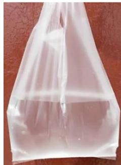
**Gambar 2.5** Contoh Plastik Jenis *High Density Polyethylene*
