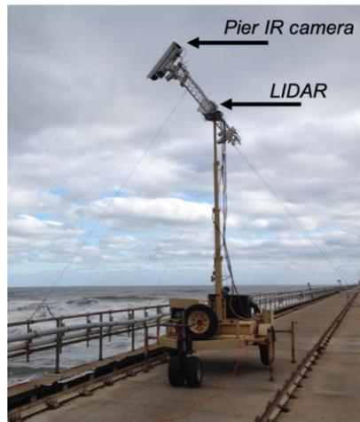
**Gambar 2.3** *Optical Wave Gauge.*
