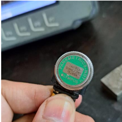
Gambar C. 13 Probe Lurus 5 MHz Diameter 0,25 inci
