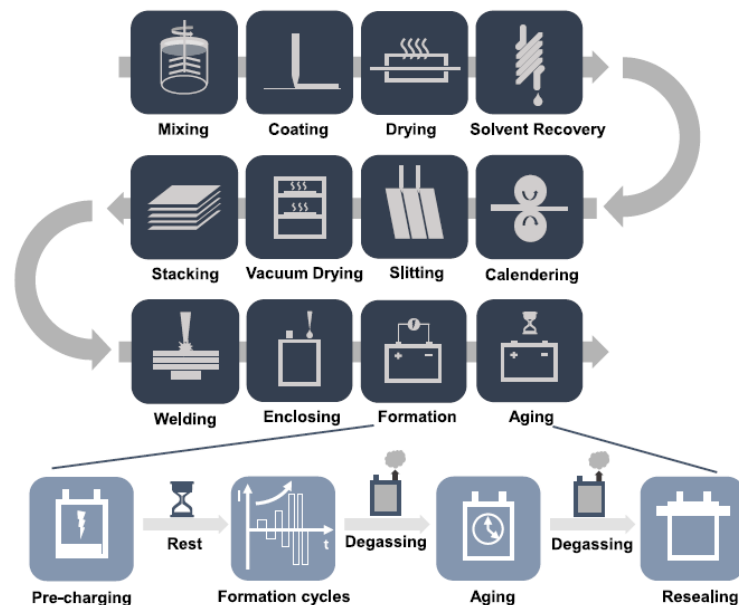
Gambar 2.7 Proses manufaktur LIB (Liu, et al., 2021)
