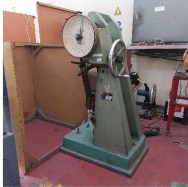
**Gambar 3.11** Alat Uji Impak
