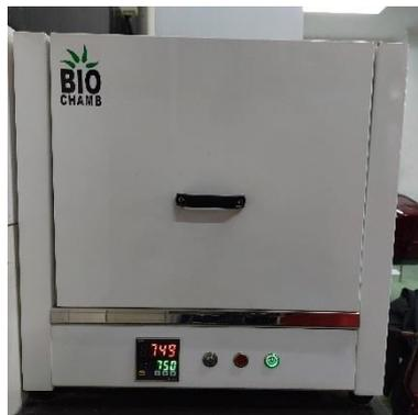
**Gambar 3.6** *Muffle Furnace*
