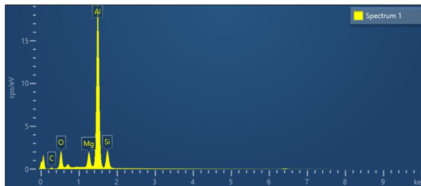
**Gambar 4.9** Spektrum EDS *Artificial Aging* 1 Jam
