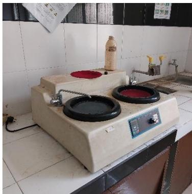
**Gambar 3.18** *Mesin Grinding Polishing*
