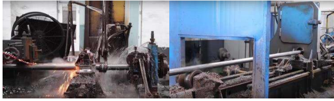
Gambar 3.2 Proses welding , quenching , dan cutting
