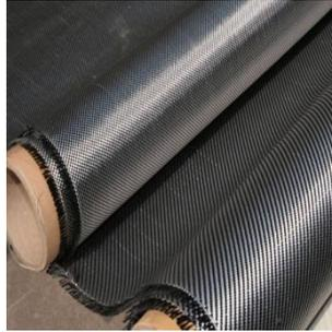
**Gambar 2.8** *Polymer Matrix Composites*
