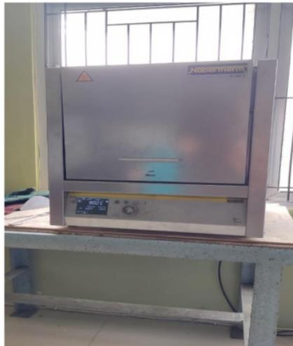
**Gambar B.4** *Muffle Furnace*
