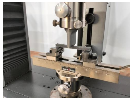
Gambar 4.4 Uji Kelenturan 3 Point Bending
