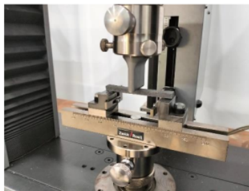
Gambar 4.4 Uji Kelenturan 3 Point Bending
