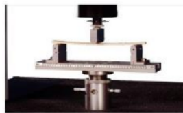
Gambar 2.4 Metode 3 Point Bending
