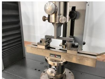
**Gambar 4.4** Uji Kelenturan 3 Point Bending
