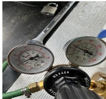
**Gambar 3.8** *Pressure Gauge* Hidrogen ( $H_2$ )
