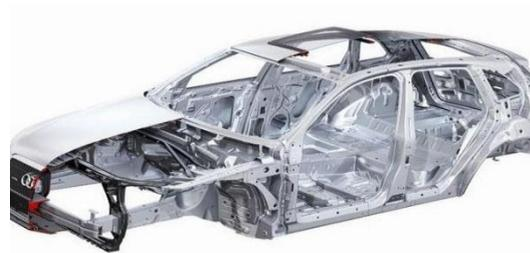
**Gambar 2.4** Rangka/*Frame*
