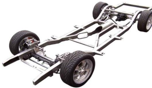
**Gambar 2.5** Rangka *Ladder Frame*
