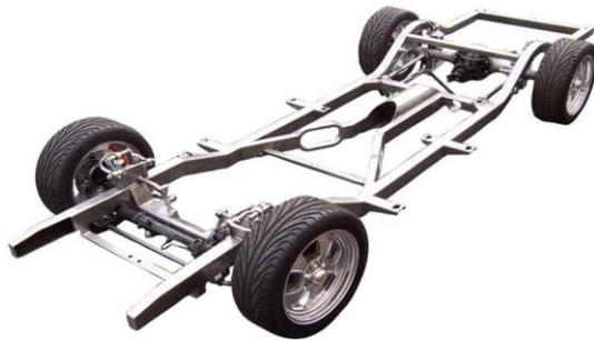
**Gambar 2.5** Rangka *Ladder Frame*
