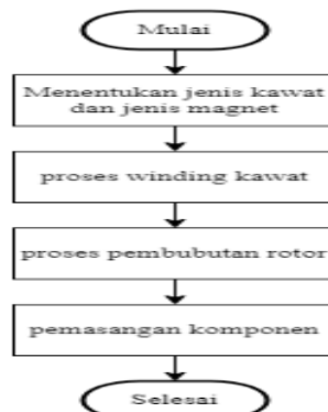
Gambar 3.3 Flowchart Perancangan GMP
