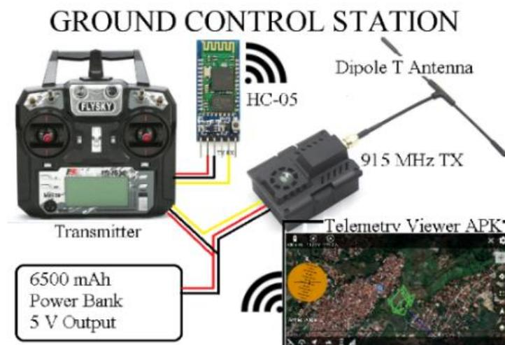
Gambar B.44 Ground Control Station (GCS)
