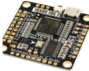
Gambar B.33 MATEKSYS Flight Controller F405-STD [24]
