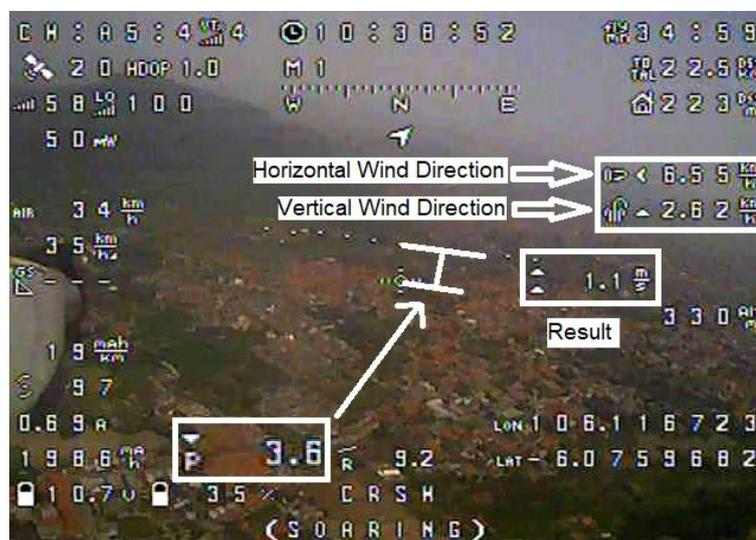
Gambar B.30 OSD Ketika Mengalami *Thermal Uplift*
