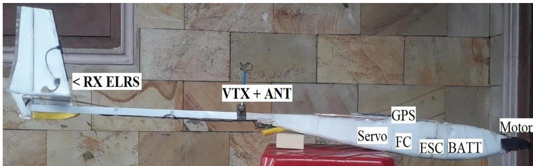
Gambar B.11 *Component Placement*
