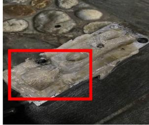
**Gambar 4.25** Cacat *Flashing*
