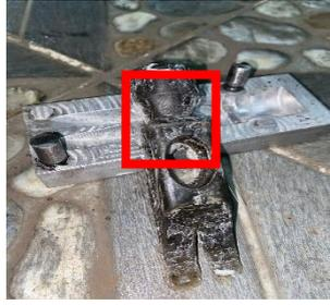
**Gambar 4.26** Cacat *Bubbles*
