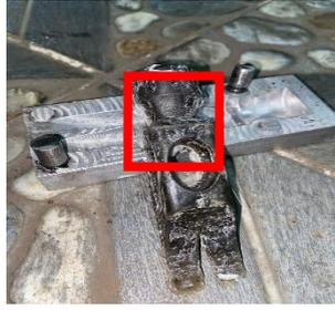
**Gambar 4.26** Cacat *Bubbles*
