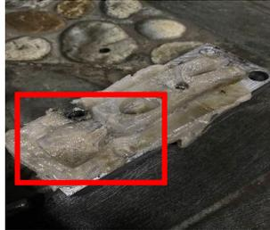
**Gambar 4.25** Cacat *Flashing*
