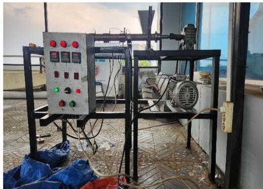
**Gambar 3.2** Mesin Injeksi *Molding*
