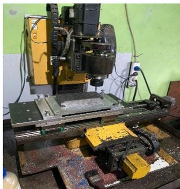
**Gambar 2.22** Mesin *CNC 3 AXIS*
