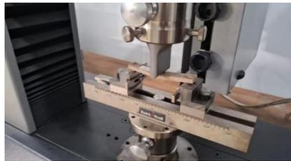
**Gambar 3.28** Uji *Modulus of Elasticity*
