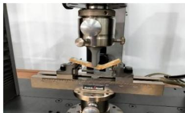
**Gambar 3.27** Uji *Modulus of Rupture*
