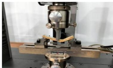
**Gambar 3.27** Uji *Modulus of Rupture*
