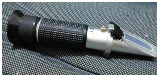
**Gambar 3.5** *Refractometer*
