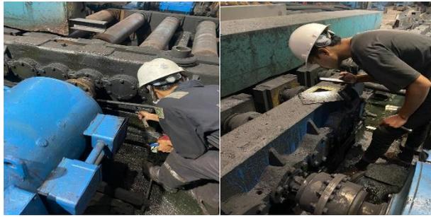
**Gambar 4.13** Pengecekan Pondasi *reducer roll table entry* dan *delivery*
