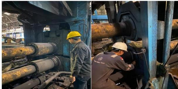
**Gambar 4.16** Pengecekan *Wobler spindle head*
