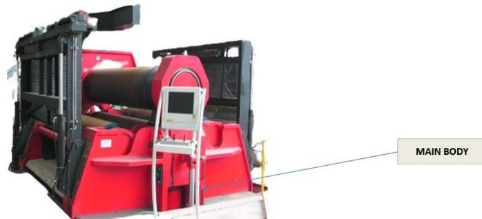
**Gambar 3.3** *Body* Mesin Roll Bending
