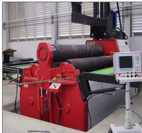
**Gambar 3.2** Mesin *Roll Bending*
