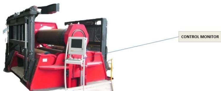
**Gambar 3.7** Control Monitor Mesin *Roll Bending*
