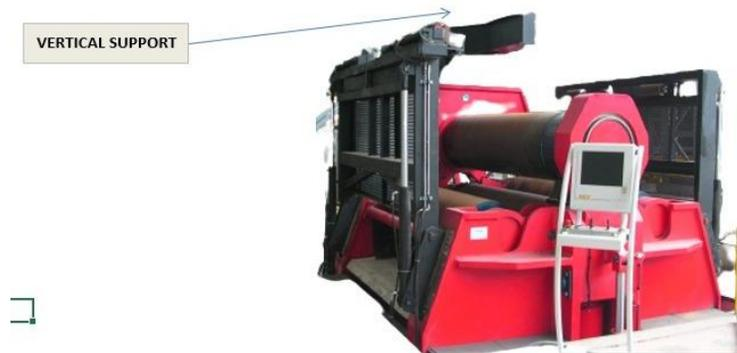
**Gambar 3.4** *Vertical Support* Mesin Roll Bending
