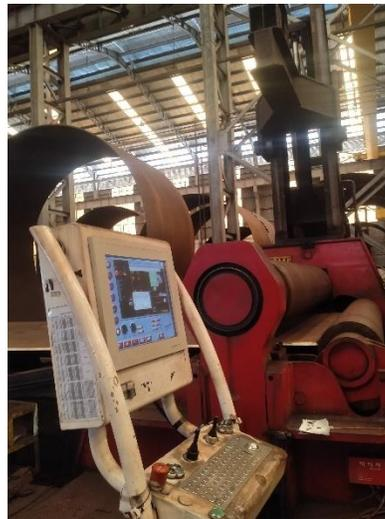
**Gambar 4.1** Mesin *Roll Bending*
