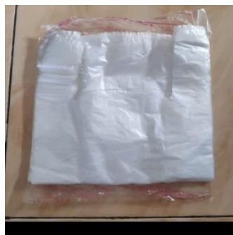
Gambar 2.6 HDPE ( High Density Polyethylene )
