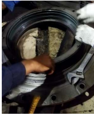
Gambar 4.7 Penggantian Oil Seal
