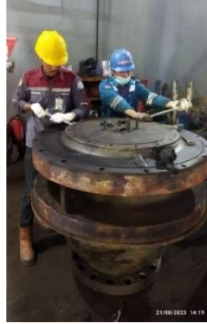
Gambar 4.4 Melepas Keeper Grinding Roll
