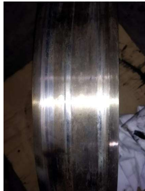
Gambar 4.4 Shaft Sleeve Terkikis
