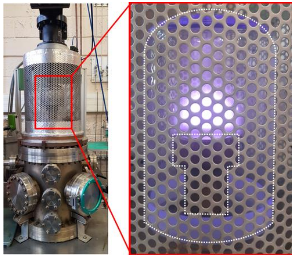
Gambar 3.2 PECVD Bell-jar Reactor [40]
