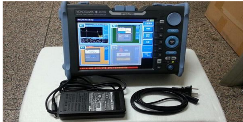
Gambar 3.7 Optical Time Division Reflectometer (OTDR) Yokogawa AQ7932
