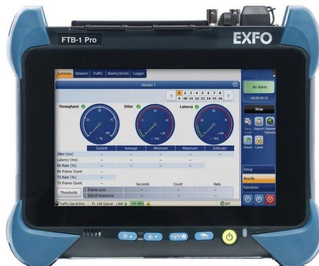
Gambar 3.8 Optical Time Division Reflectometer (OTDR) EXFO FTB-1 Pro
