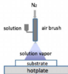
Gambar 2.2 Skema Spray Coating [27]
