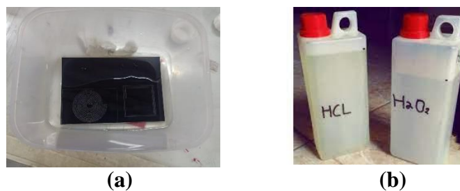
Gambar 3.18 (a) Proses etching (b) Larutan HCl dan H 2 O 2
