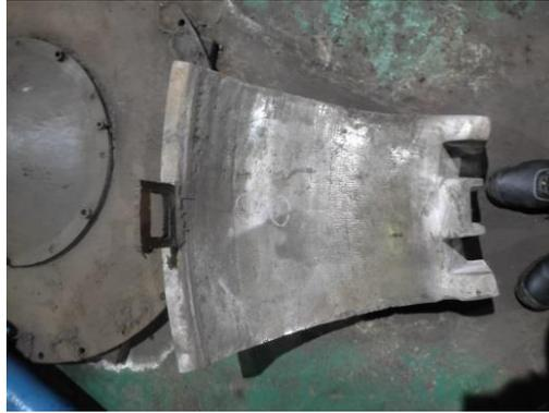
**Gambar 3.6** *Grinding Ring Segment*
