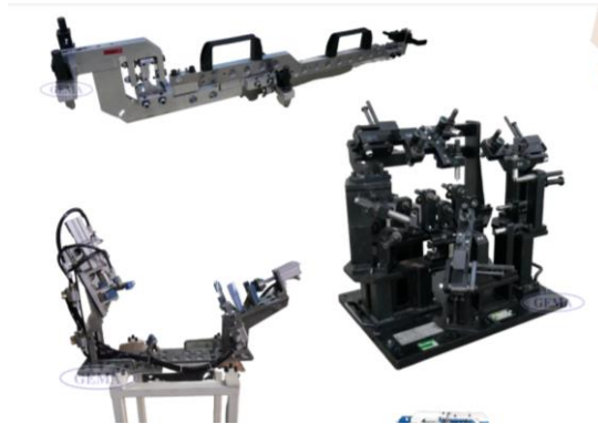
Gambar 2.4 Jig and Fixtures
